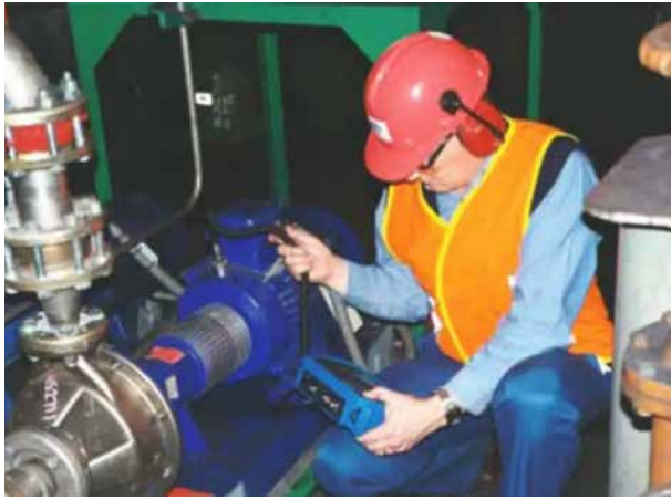
Above left: Fig.2. Technician collecting a vibration measurement. Above right: Fig.3. A thermographic image of a motor.
