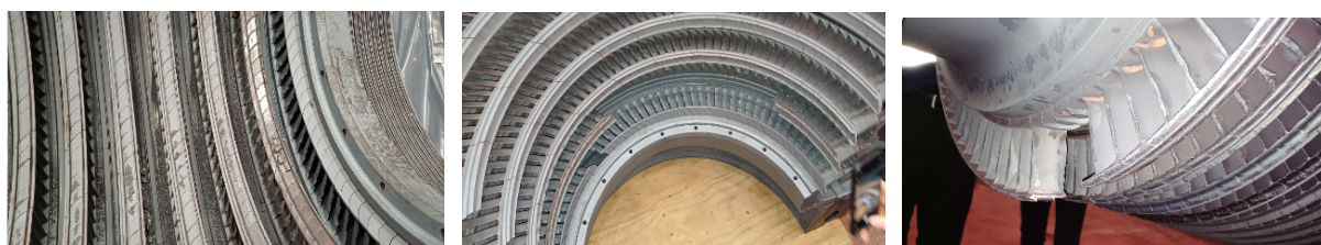
Figure 6. IP casing bottom section (left), top stationary blades (middle), IP shaft (right).
