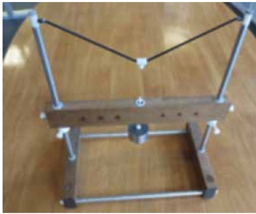
Above left: PCB Gravimetric calibrator. Above right is a screen shot from a Pico Scope when the transducer had a short free fall as described.
