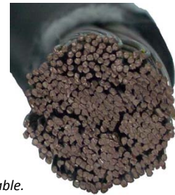
Photo 2. A 35 mm 2 crimp lug fits onto a 50 mm 2 compacted cable. (Are we right to crimp it ? Answer = NO). A 50 mm 2 crimp lug feels a bit loose on a 50 mm 2 compacted cable. (Are we right to crimp it ? Answer = YES)
