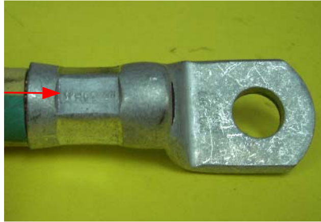
Above: The finished Crimp. Note: Crimping die Identification stamped into finished crimp ( 38-165 CU )
