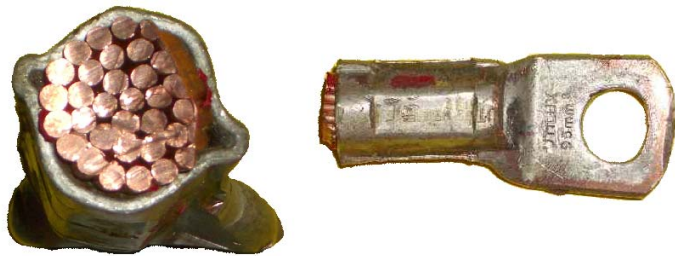
Poor Crimp – Why ? Over-crimping and tool die not aligned with lug resulting in lug damage.
