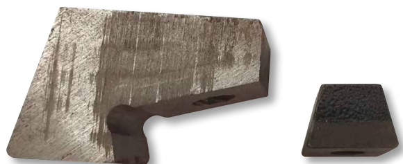
Fig. 6. Special weight on the left, standard weight on the right.
