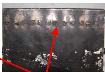
Arcing damage due to high resistance.
