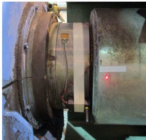
Figure 2 - Strain gauge and transmitter installation at motor shaft.
