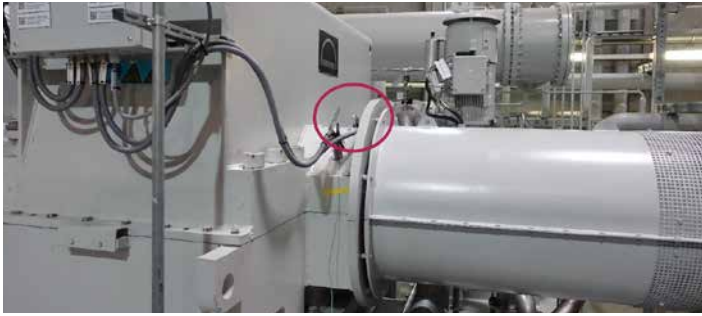
Figure 6: Accelerometer 2 on the non-drive end gear bearing in vertical direction
