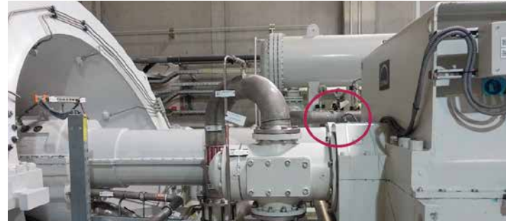
Figure 5: Accelerometer 1 on the drive end pinion bearing in vertical direction.
