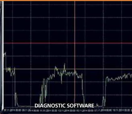
Trending of the machine vibrations to ISO 10816
