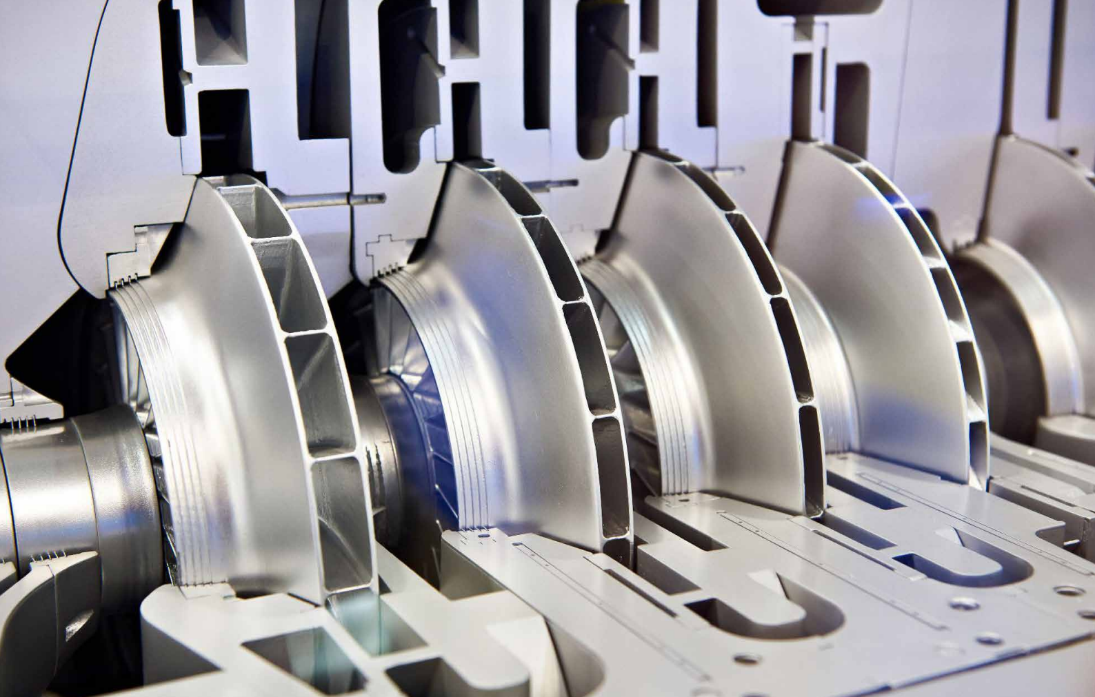
Above: A centrifugal compressor.
