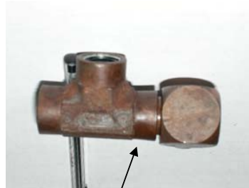
Over tightening can lead to fitting failure.
