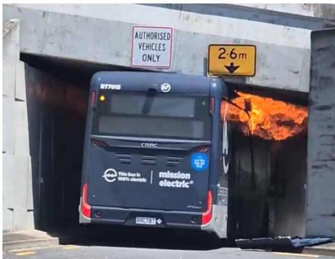
Above: Electric bus incidents demonstrate the scale of energy involved when large battery systems fail. Below: Roof-mounted bus battery systems may be exposed to weathering, impact, vibration, water ingress and corrosion.
