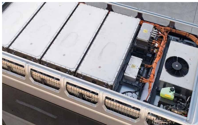
Above: Electric bus incidents demonstrate the scale of energy involved when large battery systems fail. Below: Roof-mounted bus battery systems may be exposed to weathering, impact, vibration, water ingress and corrosion.
