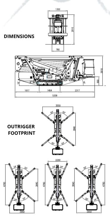
$^{\star}$  outreach and height max values and repeatability can change within  $\pm\,3\%$  due to manufacturing variation and working condition.
