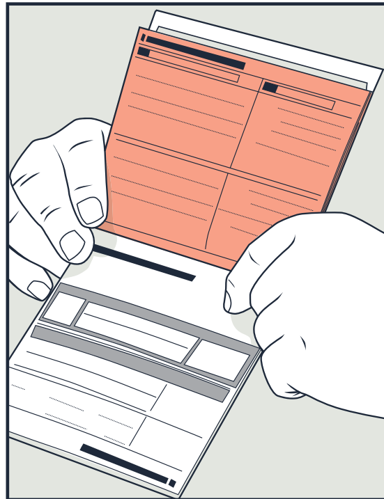
Figure 9: The operator's manual must be kept with the MEWP in a weather proof container.
