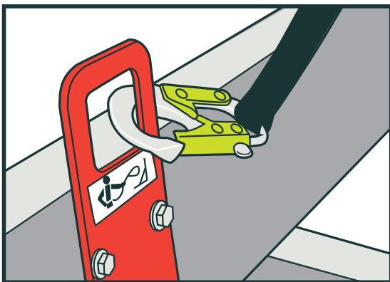
Figure 1: Attach harnesses to a certified anchor point on the MEWP.
