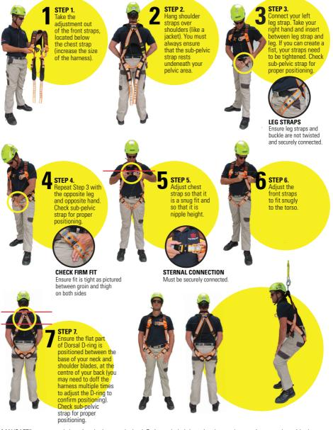
MAXSAFE® recommends hanging the harness by back D-ring to help it keep its shape when not in use and provide the worker with a starting point when next attempting to don the harness.
