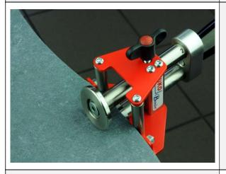
Adjust the desired bending height with the engraved scale, tighten the wing screw and insert the sheet metal between the bending wheels. The angled bending wheel will be on the inside of the resulting bend.
