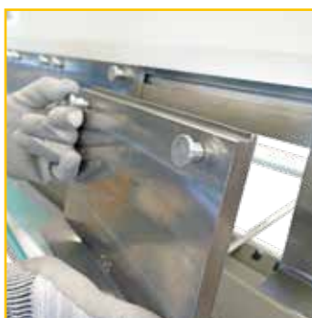
1 Quick disassembly of the segments with pull-device
