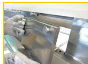
1 Quick disassembly of the segments with pull-device
