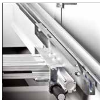
Pneumatic conical folding, manual adjustment
