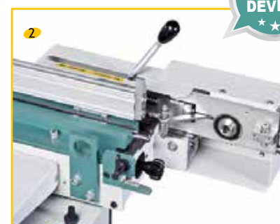
Lateral opening allows for bead removal without withdrawing the rod
