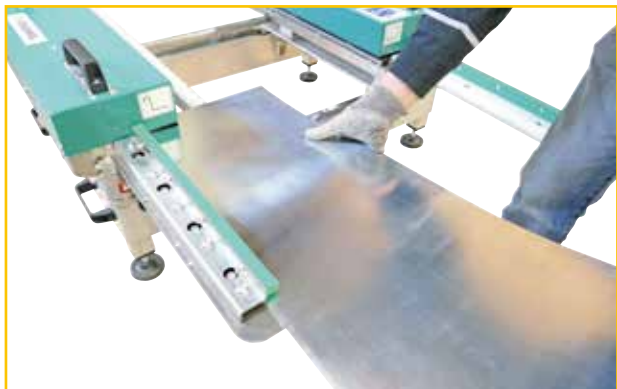
Roll-formed conical tray in 2 runs
