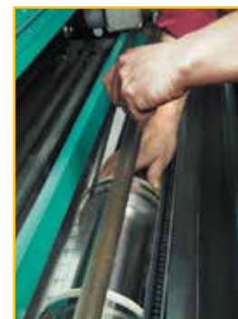
Access and quick adjustment of cutter blades
