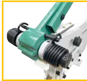
Safety: tension spring on the upper blade
