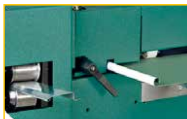
Round edge and gutter line forming
