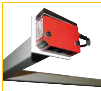
Laser control of the loop
