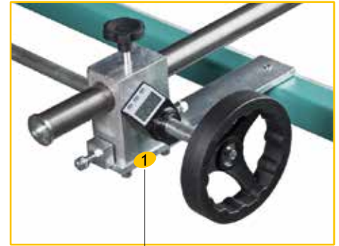
Rack-and-pinion operated back gauge, counter with digital
