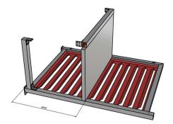
Place the shelf onto the frame so the measured 600mm is the top of the shelf and the left side of the shelf is in-line with the left side of the louvre wall frame. Fasten shelf to the frame with the supplied screws.
