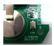
A reset button was build on the PCBA
