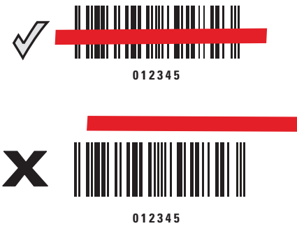
Figure 3-3 Scanning Orientation with Aiming Line
